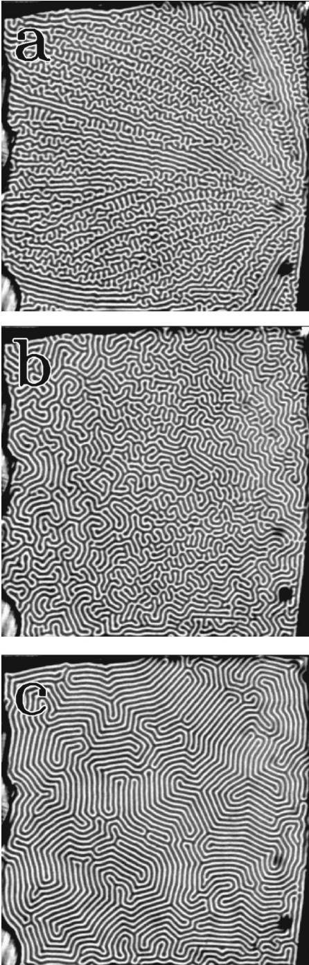
FIG. 5. Development of the domain pattern under periodic modulation according to Eq. (1) with B_0 = 1.8 mT and f_D = 1 Hz. Elapsed time (a) t = 0 s, (b) t = 50 s, and (c) t = 5000 s.
